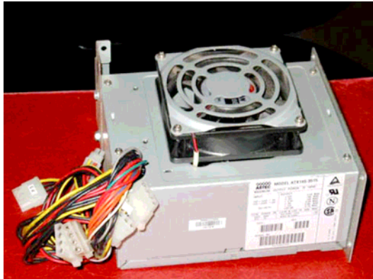
(a) Enclosed Frame Internal Power Supplies
